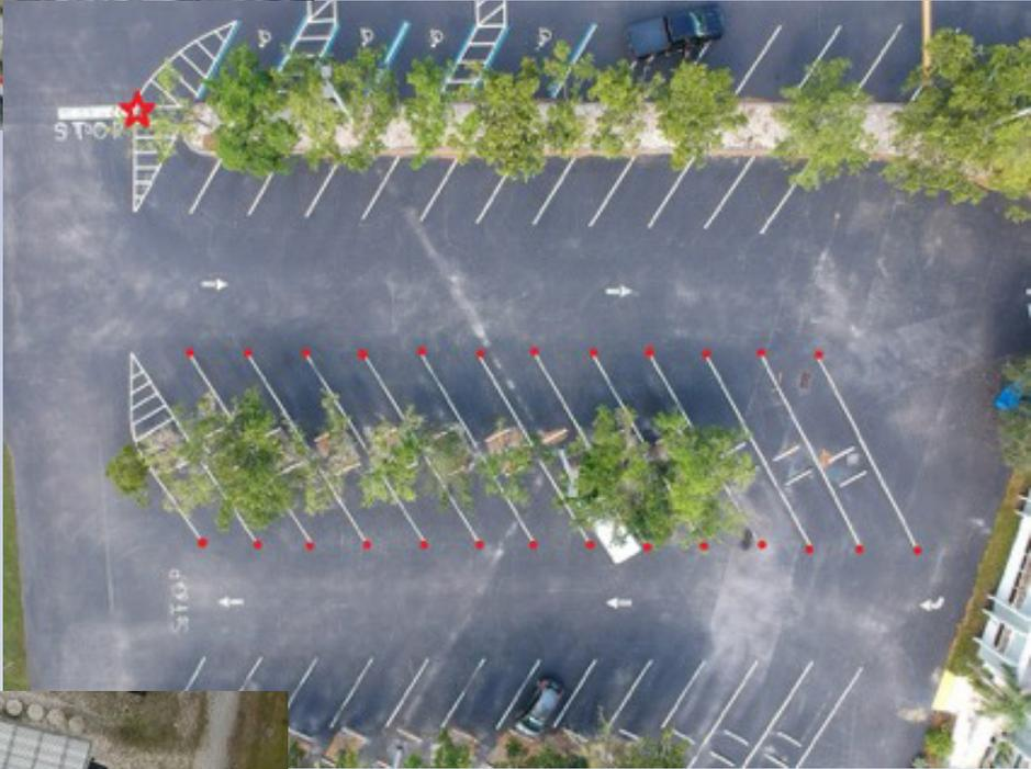
Figure 2 Broward County Extension Parking lot located at the East of the project site, provides a mixture of medium to low density trees. The red star represents one of the control points and the red dots represent the westmost corner of the paint stripe measured.
