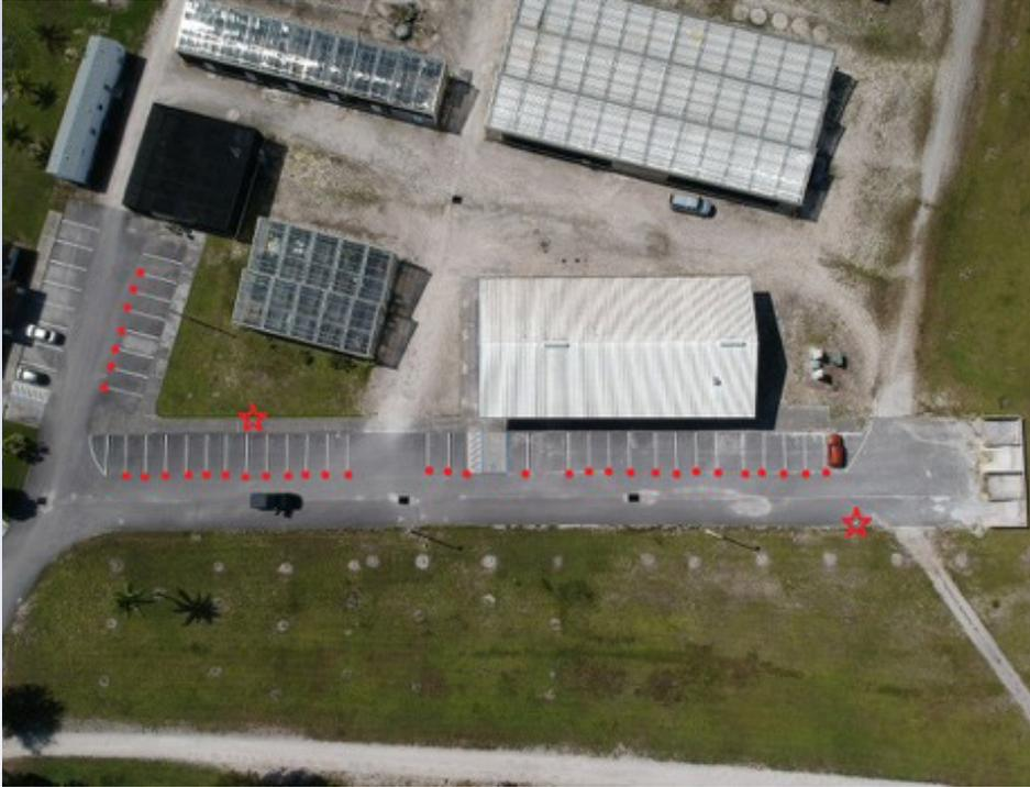
Figure 3 The Green House Parking lot located at the West of the property site. With only a one-story building serving as the main obstruction, this area provided an environment with less tree coverage than Broward County Extension Parking Lot. The red stars indicate the location of control points and the red dots the southmost and the westmost corner of the paint stripe measured.
